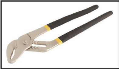
Groove joint plier or adjustable spanner.
